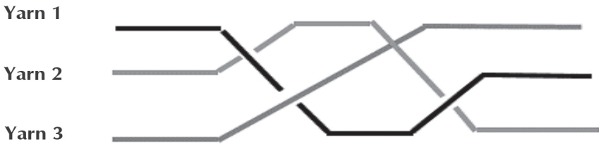
FIGURE 3.15 Path of the interlaced yarns in braided structure.
